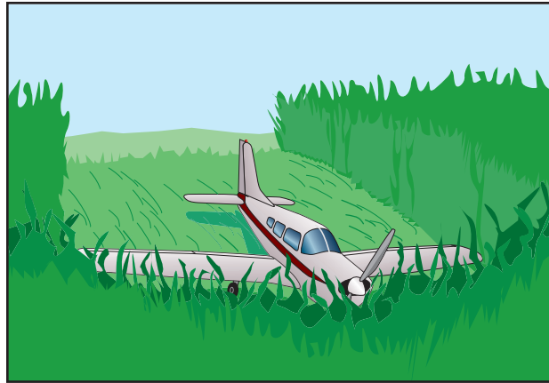
Figure 16-1. Using vegetation to absorb energy.
