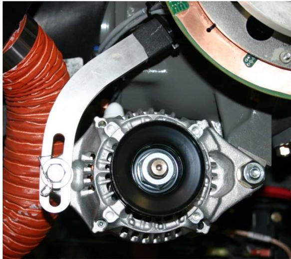
**Figure 7-33 Alternator Installation**
